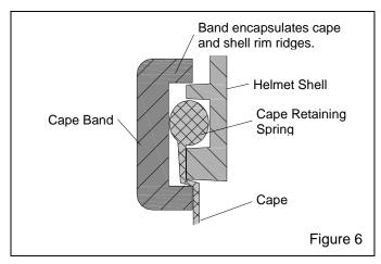
**9.4.6** Place the attachment band over the cape as shown in Figure 6. When correctly positioned, the buckle is on the window hinge side of the helmet, and the tensioning strip points toward the front.
