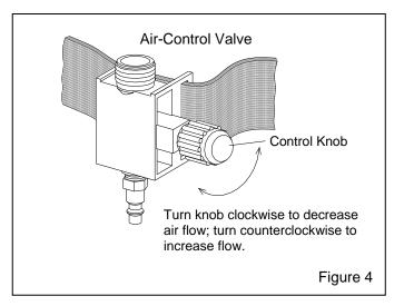
**6.2.1** Clemco's ACV air-control valve allows the user to increase or decrease the volume of breathing-air while wearing the supplied-air respirator. The valve provides a range of 7 to 10 cfm of breathing-air when the respirator is supplied with respirable air as noted in Section 4.4.
